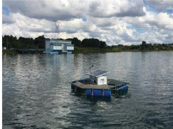
Figure 5: Measurement platform close the water intake of Passaúna reservoir.
