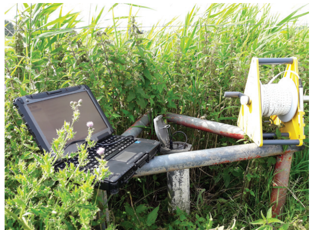
Groundwater monitoring site with data logger. The data is used to model future water balances in coastal regions.
