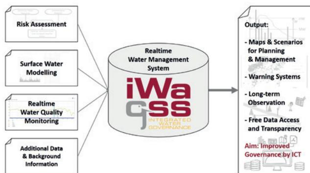
Figure 2: Components of the iWaGSS real-time water management system (Source: IEEM).
