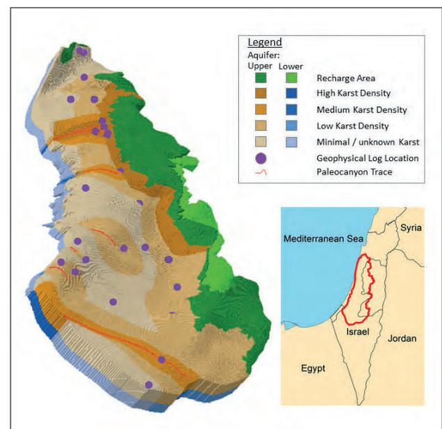
*Figure 1: Numerical Groundwater model and key karst features implemented into the stochastic modelling concept*
