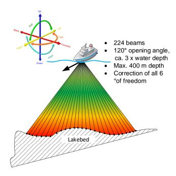
Fig. 1. Setup of the acoustic measurement system
