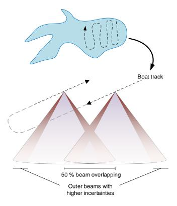
Fig. 2. Beam overlapping to increase bathymetric data quality
