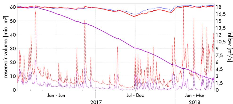
Figure 3: Comparison of two different simulations of the volume in Passaúna reservoir for the years 2017/2018. The versions differ only with respect to precipitation input (broken lines, right y-axis). In version 4, actual precipitation is reduced by 50%.
