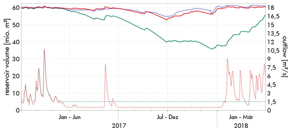
Figure 2: Comparison of two different simulations of the volume in Passaúna reservoir for the years 2017/2018. The versions differ with respect to minimum (ecological) outflow. The baseline simulation assumes a min. outflow of 0.5 m<sup>3</sup>/s, version 3 of 1.5 m<sup>3</sup>/s (total outflow as broken lines on right y-axis).
