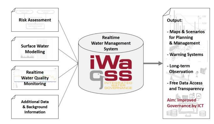
The iWaGSS real-time water management system links different tools and methods, e.g. risk assessment, surface water modelling and real-time water quality monitoring in a single data management and decision support system providing reliable and transparent information for both water managers and stakeholders.
